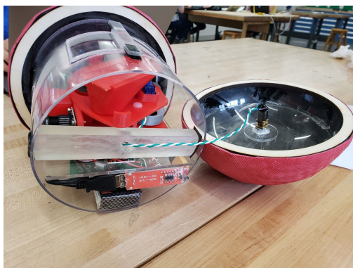
Picture of PupBuddy with left wheel removed, showing a strut and the electronics
